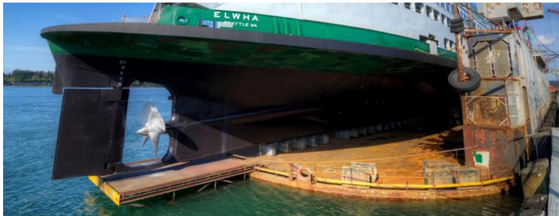
Figure 16 Conventional propulsion arrangement: fixed-pitch propeller with flat-plate rudder (© Sol Duc Photography)
